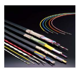
SPEC 55 wire is insulated with modified radiation cross-linked ETFE polymer. It has a temperature rating of -65°C to 200°C [-85°F to 392°F] continuous using a silver plated copper conductor, and combines the easy handling of a flexible wire with excellent scrape abrasion and cut-through characteristics.
